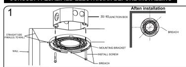
Hold Mounting Bracket up to junction box with flange facing down. Align breach side of the Mounting Bracket parallel to nearest wall. Screws mounting bracket to j-box.
