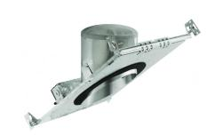
ELCO Slant allows for installation in sloped ceilings ranging from 7/12 (30°) to 12/12 (45°). Can be used in insulated ceilings. Fits in 2" x 8" joist construction.
