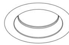
Regressed Reflector Trim with Frosted Lens 4 7/8" O.D.
