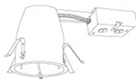
3" Standard ICA Housing 750 lm (10.5W) w/ELK19 Series Module 950 lm (10.5W) w/ELK21 Series Module Remodel
